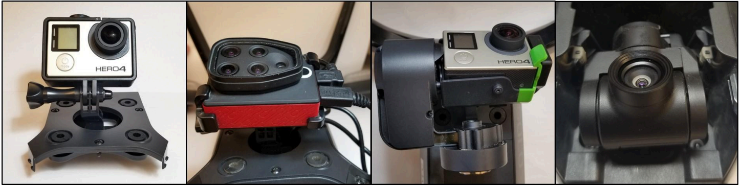
Figure 3: Mounted cameras that face the same direction during the flight (a,b) are not as useful for scouting as those on a rotating gimbal (c,d) that you control from the ground. (Photos: Jarrod Miller)
