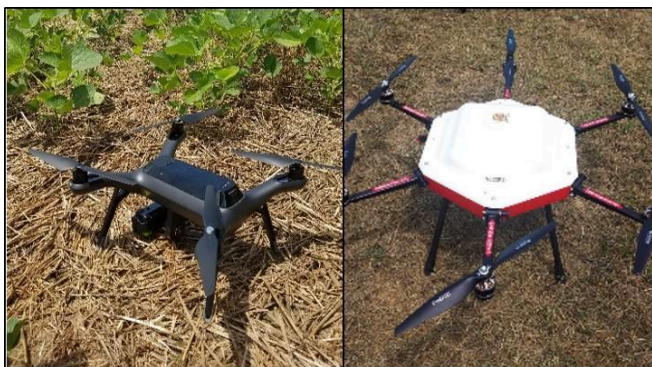
Figure 1: A quadcopter (left) versus a rotary with six propellers (right). (photo: Jarrod Miller).
