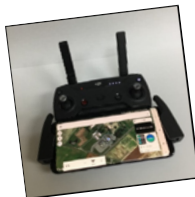
Figure 4: Controller connected to cellphone. Many newer drones have screens on their controllers.
