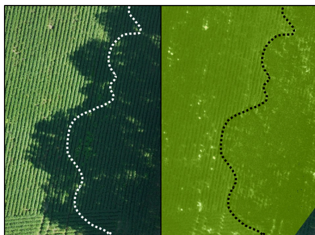
Figure 6: On the left are tree shadows in a visible image, creating patterns in the NDVI image on the right, which takes up a smaller portion than the shadow cast in the visual image.
