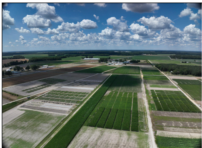
Figure 1: Cumulus clouds cast variable shadows across field plots in Delaware. These shadows affect the light reflected from plants back to cameras or sensors, causing differences across plots not related to crop growth (photo: Jarrod Miller).
