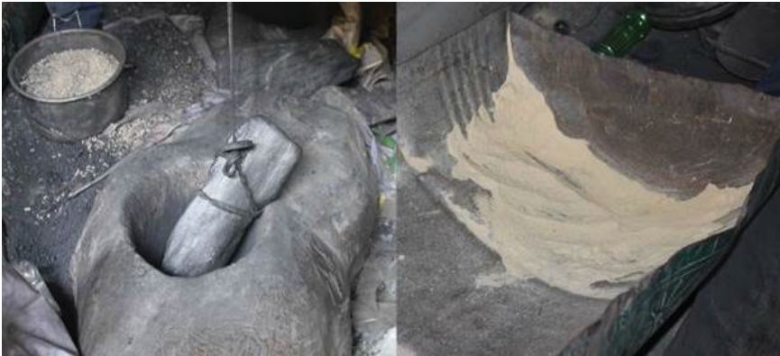
Figure 6. The sedo is ground with a large stone mortar and pestle (left) to a fine powder (right). The ground sedo is then mixed with the ground black clay (Y. Xu).
