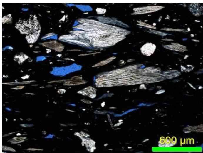
Figure 21. In thin sections of fired sherds, especially those fired below 1000°C, there is enhanced parting and splitting between layers of some of the talc particles that occurs with loss of water of hydration. These underfired talc particles are friable until fired at a temperature above 1000°C (C. L. Reedy).
