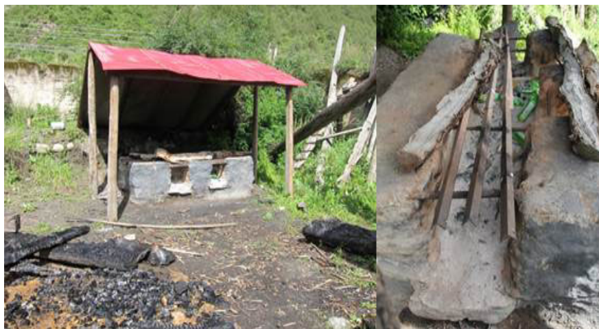
Figure 12. Kiln (left) with slots for inserting pine wood fuel, and firing trench with metal grate (right) where pots are placed during firing; piled charred wood at lower left marks the location of the second kiln, a pit kiln that fires to a higher temperature (C. L. Reedy, left; Y. Xu, right).
