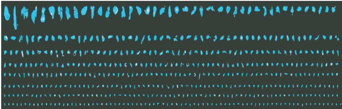
Figure 2. Here pores are sorted by size (length/ferret diameter). This type of image is useful for examining the range (here we see that most pores are very small), for deciding on cut-off points for certain measurements, and for making decisions about data collection and analysis strategies.
