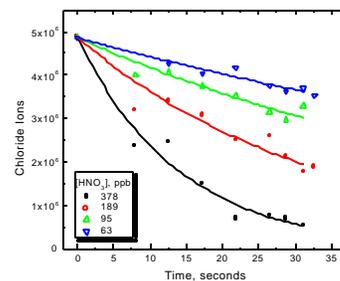
**Figure 4** displays the change in chemical composition of the aerosol as a function of contact time and nitric acid concentration in the reactor. The measured loss rate of NaCl (molecules/cm<sup>3</sup>/sec) is:
