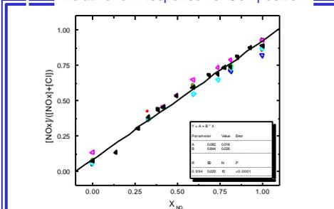
**Figure 3** demonstrates the linearity of response for internally mixed binary NaCl/NaNO<sub>3</sub> aerosols.
