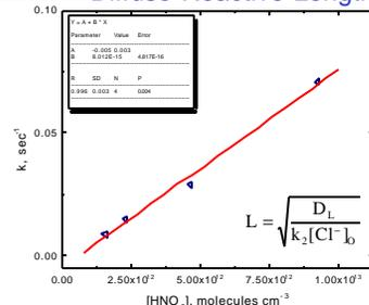
**Figure 5** shows the dependence of the rate coefficient on nitric acid concentration. The diffuso-reactive length is a parameter used to describe where the reaction takes place in the droplet. By calculating the  $[\text{Cl}]_0$  in the droplet, it can be computed.<sup>4</sup> In this case  $L = 4$  nm for  $d_p = 100$  nm.
