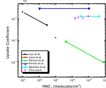
**Figure 6** shows the reactive uptake coefficient for HNO<sub>3</sub> on NaCl from different laboratories as a function of [HNO<sub>3</sub>].<sup>4</sup>
