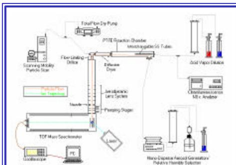
**Figure 1** is an illustration of the experimental apparatus. The change in particle composition is monitored with a single particle TOF mass spectrometer. Nitric acid vapor reacts with sodium chloride droplets in the flow tube reaction chamber. Kinetic runs are performed as a function of nitric acid concentration and contact time.
