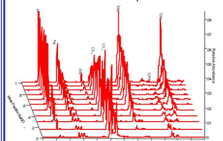
**Figure 2** shows the response of the mass spectrometer to particles that were prepared with different known chemical compositions. It should be noted that for the analysis, ion intensities from individual spectra are measured and then averaged to calculate their response, shown below.
