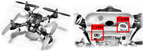
Fig. 4: Overview picture of the MAV (top). The camera configuration with the frontwards camera (CAM0) and downwards facing camera (CAM1) are shown in the bottom.
