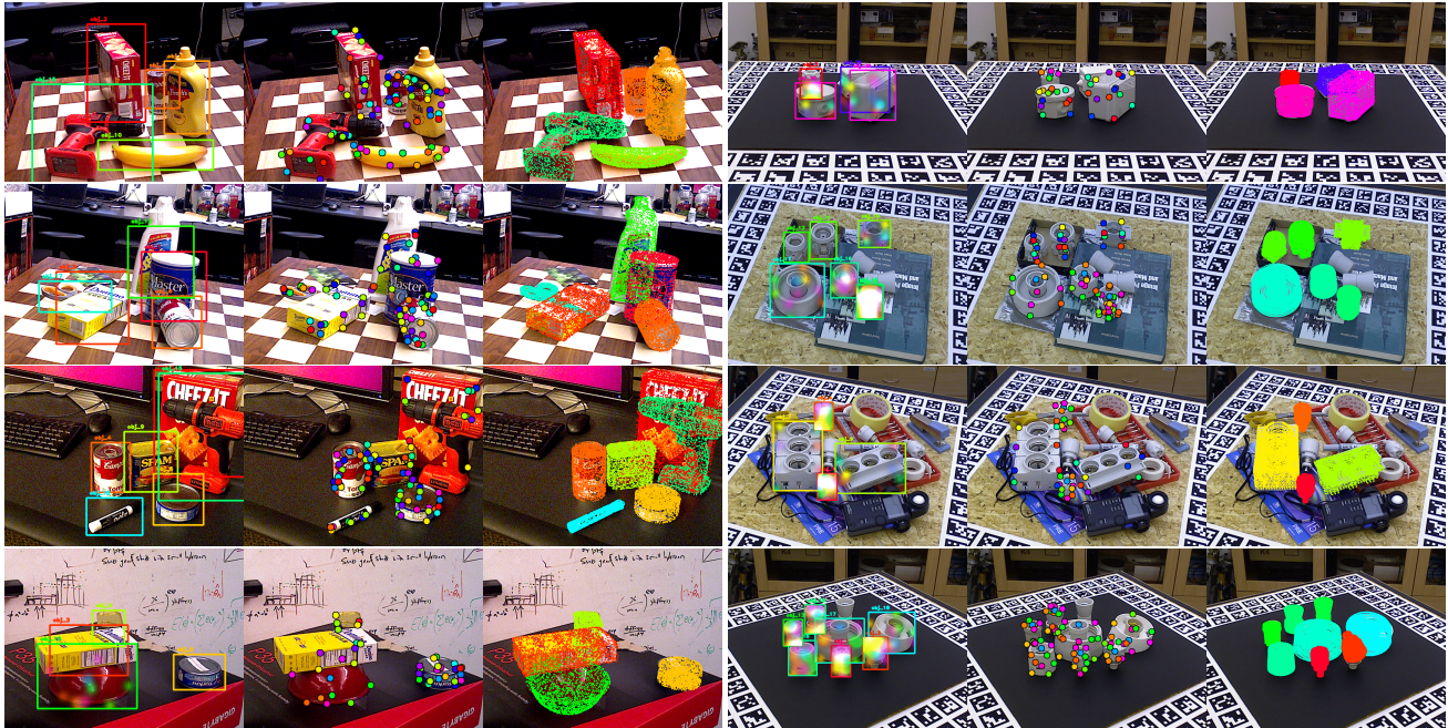
Figure 10. Supplementary qualitative results for the YCB-Video (left) and T-LESS (right) datasets. The top three rows show some successful pose estimates from our system while the bottom row shows a failure case. The failure in both cases is from initializing objects upside down. The bowl on the bottom left and the orange object on the bottom right is upside down while the are upside down.
