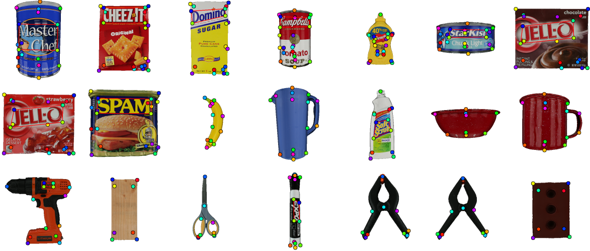
Figure 8. Our keypoint labels for the YCB-Video dataset. We labeled identifiable features based on the shape class of the objects (box-like, cylinder-like, and hand tool) which are common within different instances of the same shape class (such as box corners, cylinder top/bottom center, etc), and then instance-specific keypoints of other identifiable features such as brand names, bar codes, etc.
