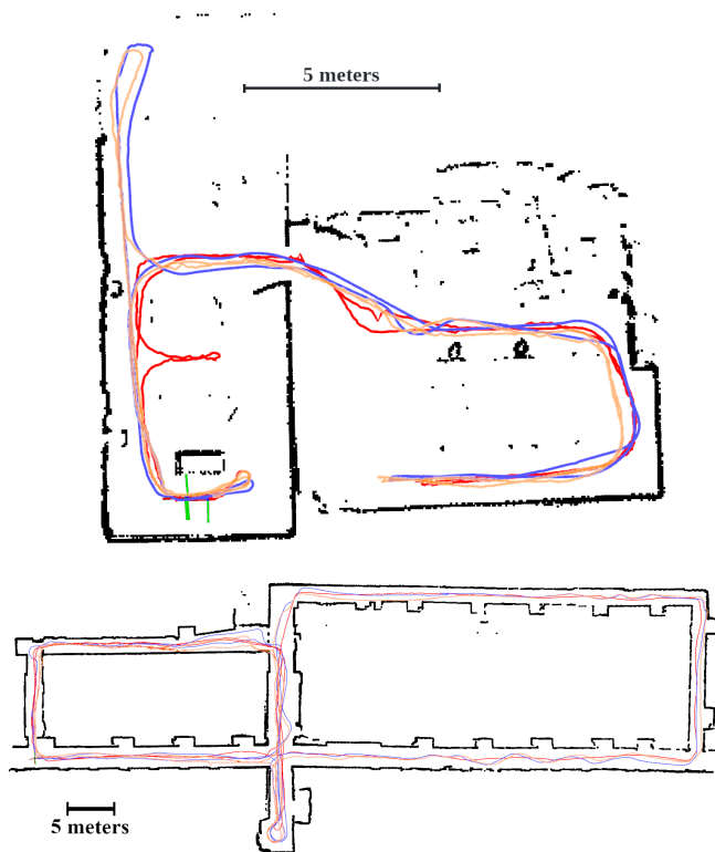
Fig. 5: A two room (top) and building floor (bottom) datasets collected with a Turtlebot3. Each map and the mapping trajectory (red) was used by the localization system (blue) on a second dataset through the environment. The batch optimized trajectory (orange) of the second dataset can also be seen.
