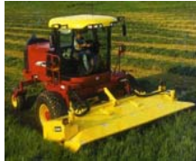
Conventional steel shielding on the side of a Self-Propelled Windrower header.
