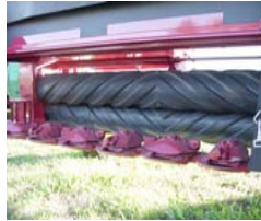
Intermeshing counter-rotating conditioning rolls on a CNH disc mower.
