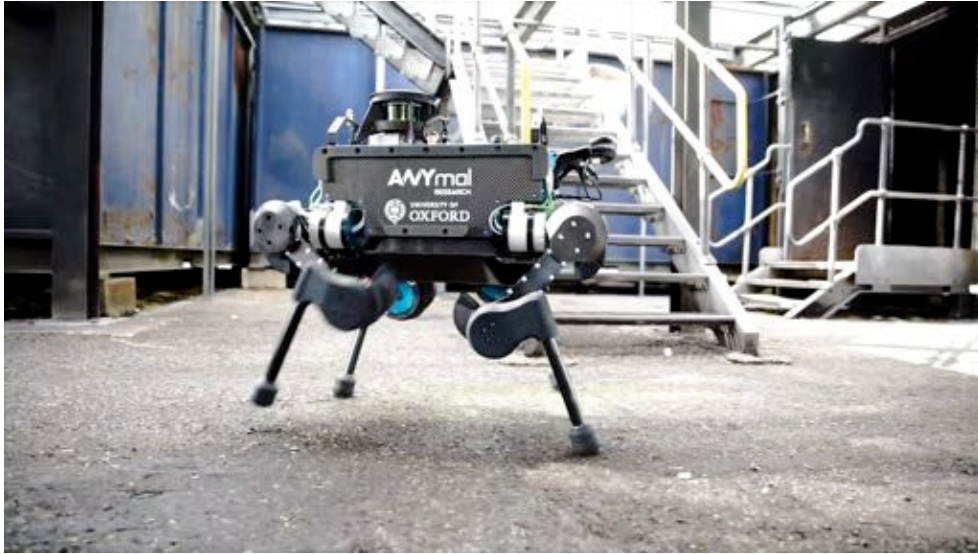
Dynamic Walking – at 0.5m/sec on Flat Ground Precise Estimate Not Important
