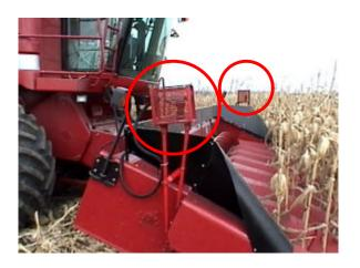
Figure 6: The head mounted cameras
