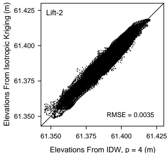
**Fig. 7:** A comparison of predicted elevation values determined using isotropic kriging and an IDW approach with  $p = 4$  (lift 2).
