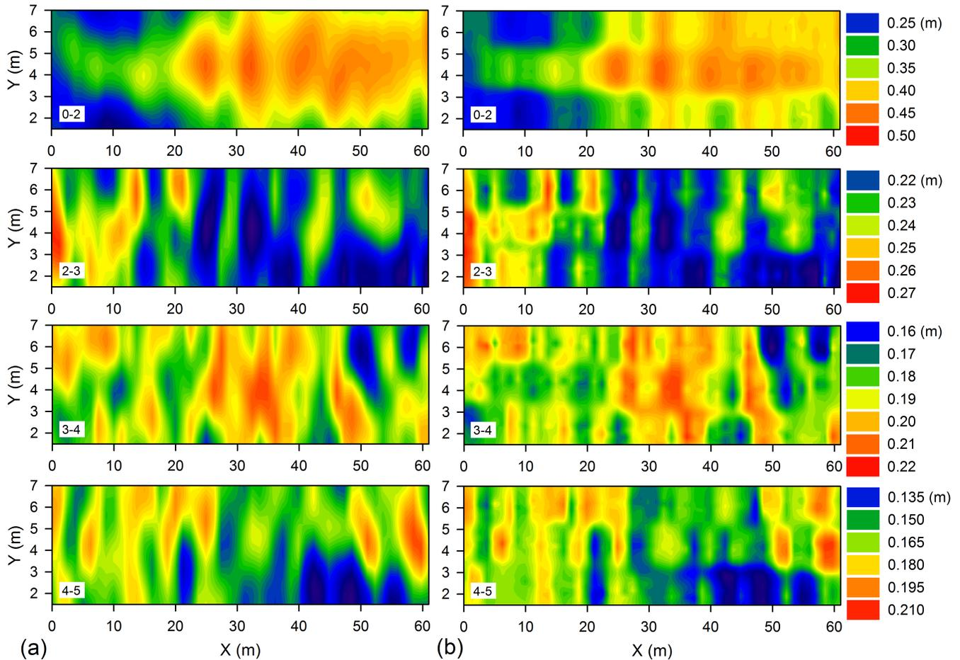
**Fig. 8:** Contour plots of lift thickness: (a) determined from elevation values interpolated using an isotropic kriging approach, and (b) determined from elevation values interpolated using an IDW approach with  $p = 4$ .
