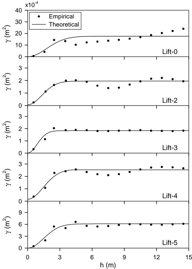
**Fig. 5:** Empirical omnidirectional semivariograms with fitted theoretical Gaussian models.
