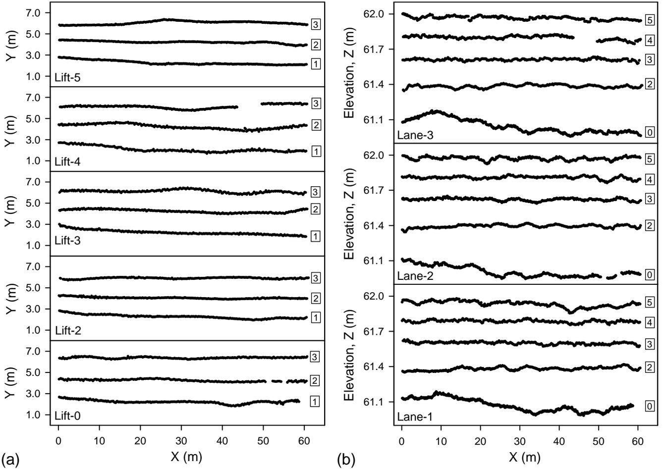
**Fig. 1:** RTK-GPS data measured by CCC equipment for five overlying lifts of compacted soil, with three lanes of compaction for each lift: (a) plan view, and (b) profile view.
