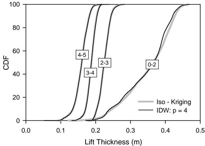
**Fig. 9:** Cumulative distribution functions showing the variation in thickness of the compacted soil layers. Results are presented for interpolation using isotropic kriging and inverse distance weighting with  $p = 4$ .
