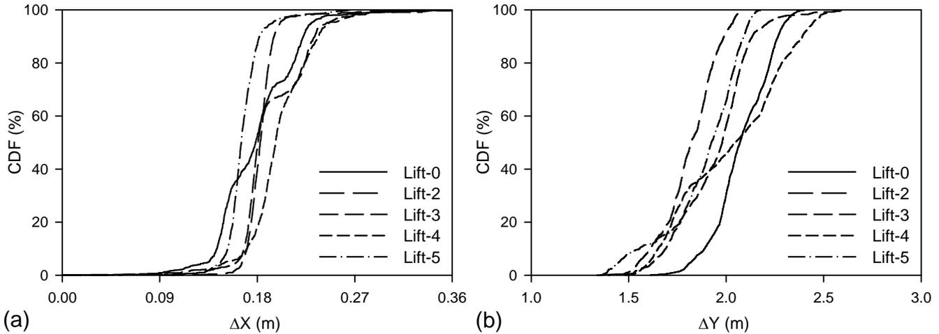
**Fig. 2:** Cumulative distribution functions of the point-to-point spacings for five lifts of compacted soil, for data collected in the: (a) X direction, and (b) Y direction.
