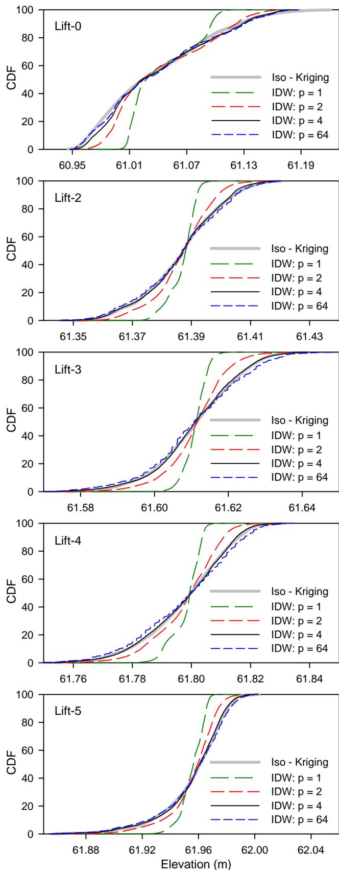
**Fig. 6:** Cumulative distribution functions of the predicted grid point elevation values for five lifts of compacted soil. Results are presented for interpolation using isotropic kriging and inverse distance weighting with different  $p$  values.
