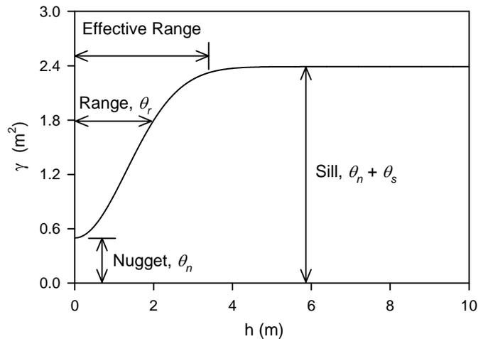
**Fig. 3:** A typical Gaussian theoretical semivariogram.
