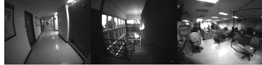
Figure 6: Selected views during the night multi-floor trajectory show the high noise, poor lighting conditions, and motion blur that greatly challenge visual feature tracking.
