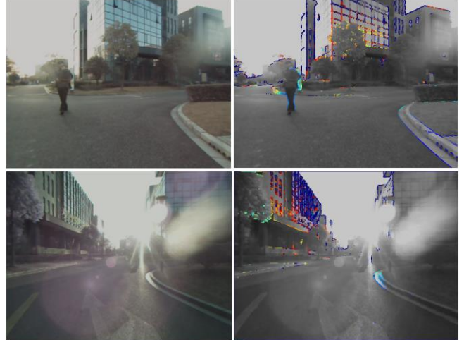
Figure 5. Images from the real experiment (upper row: dynamic people, bottom row: sudden change of light) with depth estimates. Left is rgb image, then convert to grayscale, with color-coded depth estimates are shown on the right.
